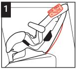
Connect and tighten harness straps prior to installing in vehicle. Place child restraint rearfacing in the back seat. With child restraint in the most reclined position, make sure level lines on shoulder belt positioning guide are level with ground. Adjust child restraint if needed.
